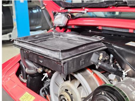
Loosen both marked hose clamps and disconnect the hoses from their fittings. Remove the four 13mm hex screws.
