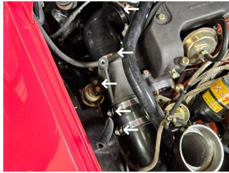
Carefully disconnect the vacuum hose from the SAI valve T-fitting. Remove the two 10mm hex screws and move the SAI valve aside. Unplug the cable connector for the boost pressure sensor.
