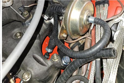
Remove the following components from the by-pass valve housing:
