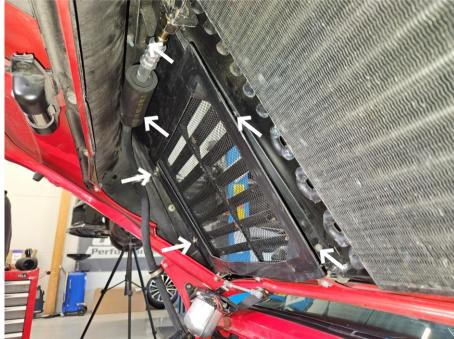
Remove the hose coupler from the turbo inlet pipe, auxiliary air valve hose, and bypass valve vacuum hose.
