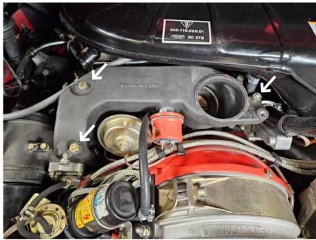
Loosen the three marked hose clamps and disconnect the hoses from their connections.
