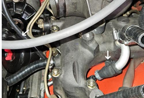
Loosen the air filter box—removal is not necessary. Loosen the two 10mm hex screws and the 13mm hex nut. Also, loosen the marked hose clamp and disconnect the hose. The air filter box must be loose to allow for the installation of the do88 intercooler.
