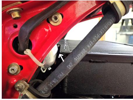
Carefully and slowly lower the deck lid (without fully closing it) and use a flashlight to check the clearance between the AC condenser tubes (on its left side) and the topright corner of the intercooler.
