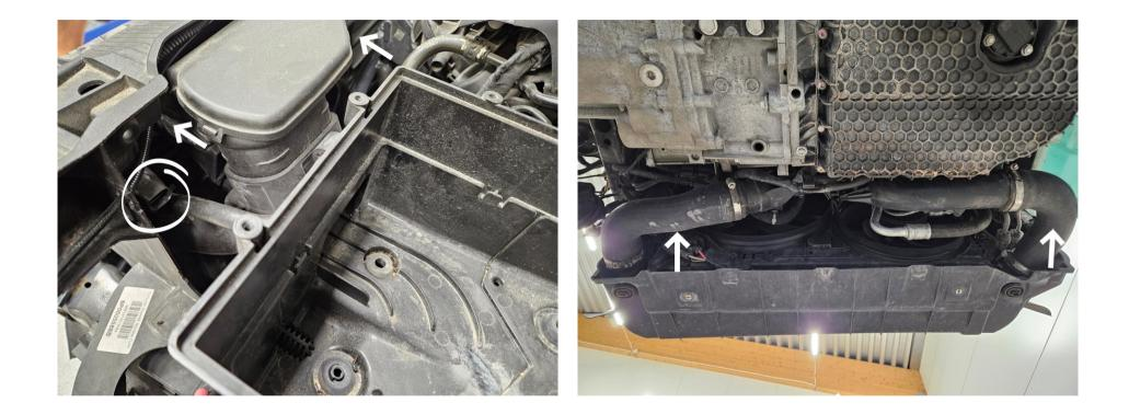
Remove the 2x T20 screws holding the airduct (marked with arrows in picture) and remove it from the car. Then disconnect the hood latch sensor.
