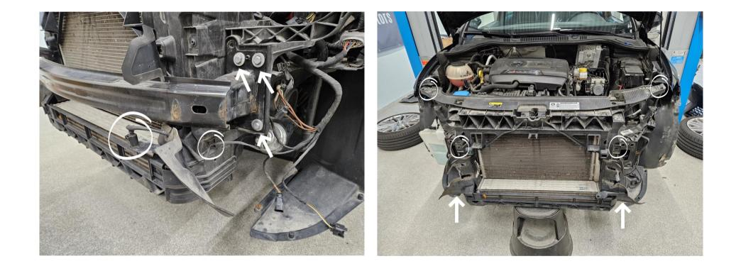
Remove the temp sensor from the radiator support. Support the radiator support and remove 6x 13mm hex screws (three on each side) then remove the bumper beam.
