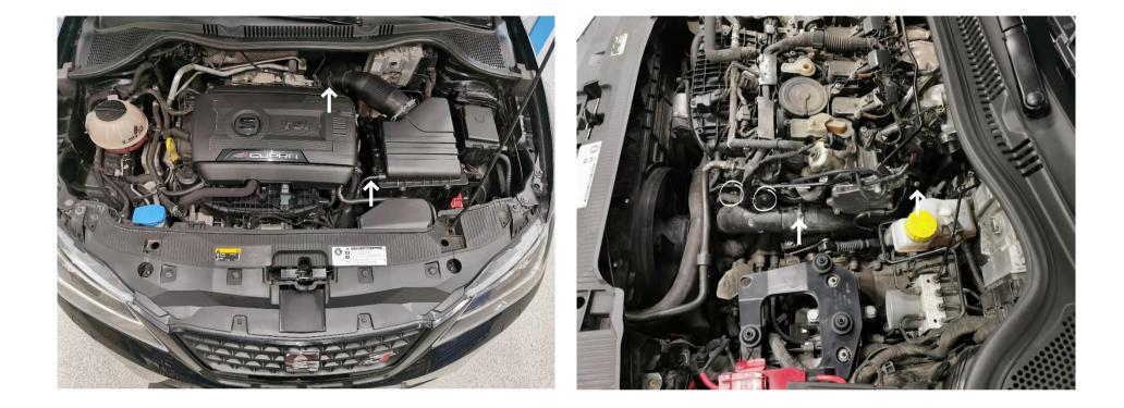
Disconnect the vacuum hose from the airbox. Loosen the rear spring clamp on the inlet hose and disconnect it from the turbo inlet elbow. Remove the airbox from the car by pulling the rear end upwards and then separate it from the front air duct. Be aware of the drainage pipe underneath the airbox.
