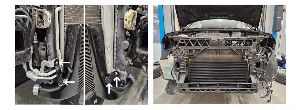
Loosely install the brackets to the intercooler with the included M6x12 4mm allen screws then lift it in place so that the radiator stands in the radiator seats in the intercooler and secure it to the AC condenser and radiator with the two T30 screws removed in previous step. Before tightening all 4 screws, make sure there is space between the intercooler and the AC-condenser.
