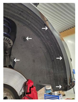
Remove the 5x T20 screws to loosen the front part of the inner wheel arch on both sides.
