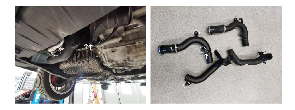
Disconnect the electrical connector from the sensor and loosen the 3x T30 screws then remove both pressure pipes downwards. The turbo to intercooler pipe can be removed both upwards and downwards.
