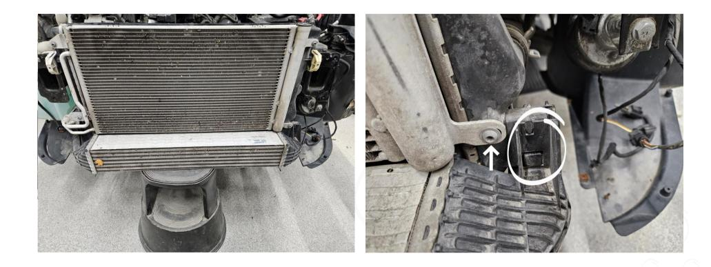
Lift the radiator support and the radiator package and while holding them both tilt the core support forwards and tilt the radiator package backwards then lift the radiator package and lower the core support to separate them. Put the core support on a support to the left minding the hood latch cable. Place the radiator package on the support previously used for the whole assembly.
