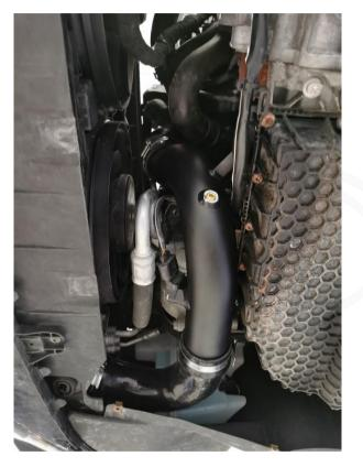
Now re-install the do88 parts in the reverse order the OE parts came out and tighten the hose clamps to 5Nm.
