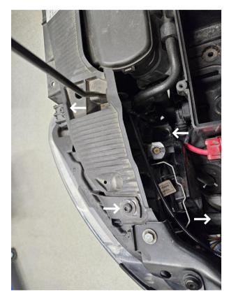
Remove the headlights by undoing 5x T30 screws on both sides (four marked in the picture and the fifth is accessed from the outside below the fender. Then disconnect the electrical connector remove the headlights from the car.
